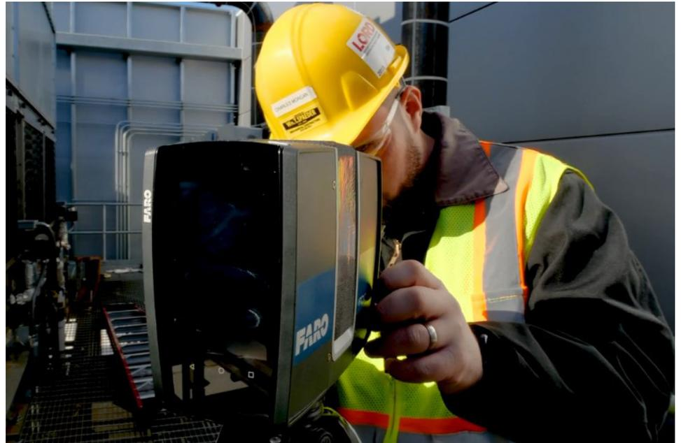
To accurately capture conditions at the Erie Insurance headquarters, mechanical contractor Wm. T. Spaeder turned to the FARO Laser Scanner.
